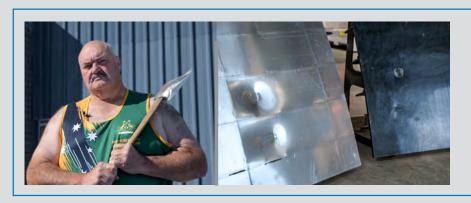
World Champion axeman, David Foster OAM took a swing at HDPE. Using similar force and the same equipment the aluminium section buckled significantly and came close to tearing. Apart from scuff marks, the HDPE was totally undamaged.
